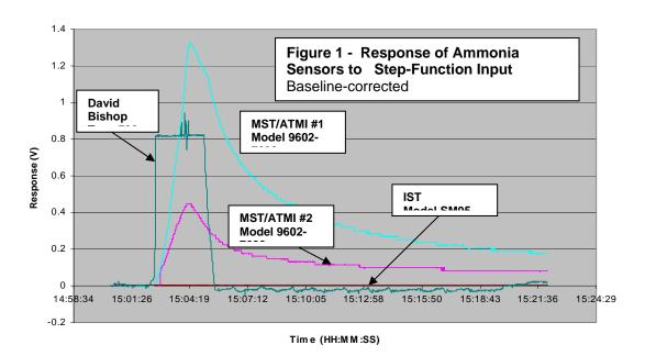
commercially-available ammonia sensor systems suitable for reliable CA monitoring (David Bishop Type 730 and the MST/ATMI 9602-200). The prototype optical ammonia sensor system under development by Pacific Technologies also appears to be a viable option assuming it becomes commercially available. Note that Industrial Scientific has chosen to *discontinue development* of its (successful) optical ammonia sensor technology for the ammonia refrigeration market.
