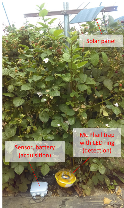
Figure 7: Field deployment of the sensors monitoring for SWD
