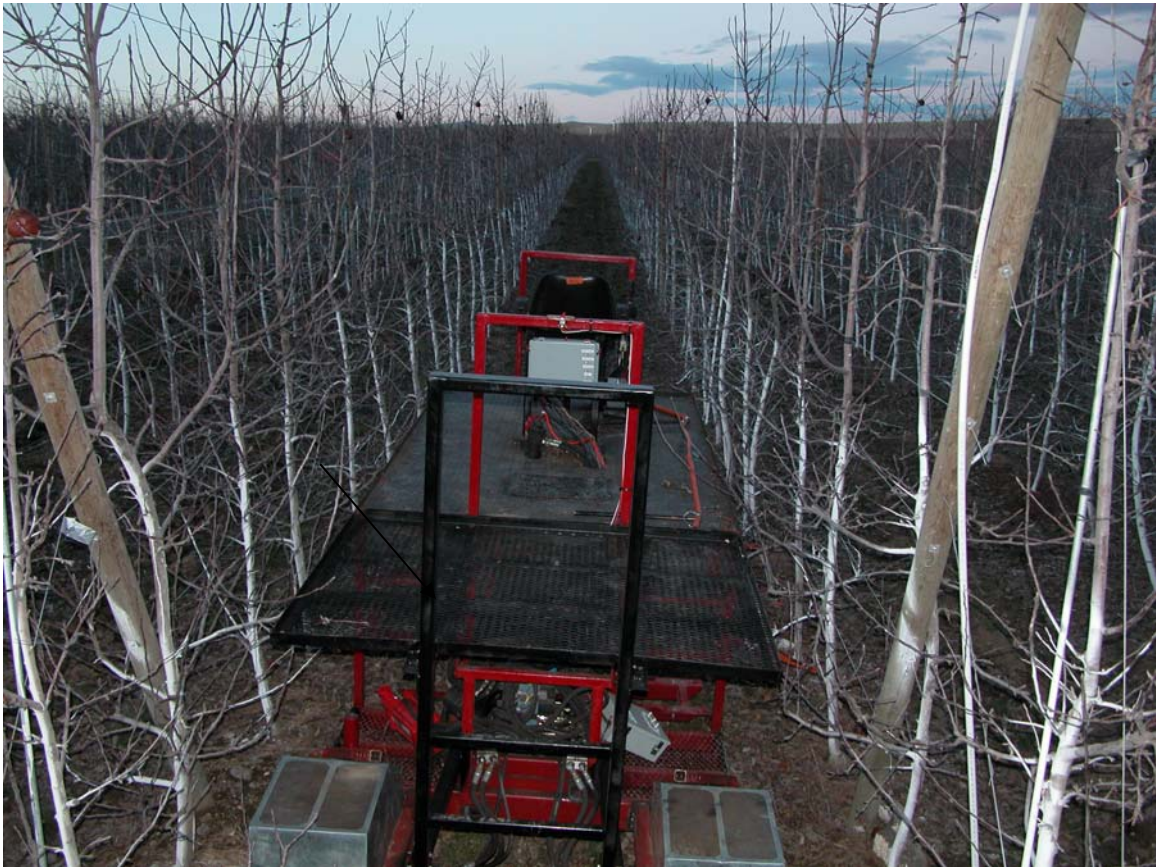
Figure 1. The modified Peterson machine with fruit handling system removed. Major modifications have been made to the worker platform, wheelbase, autosteering, and row sensing electronics modified. The machine is in an 8.2 foot wide unpruned gala row.
