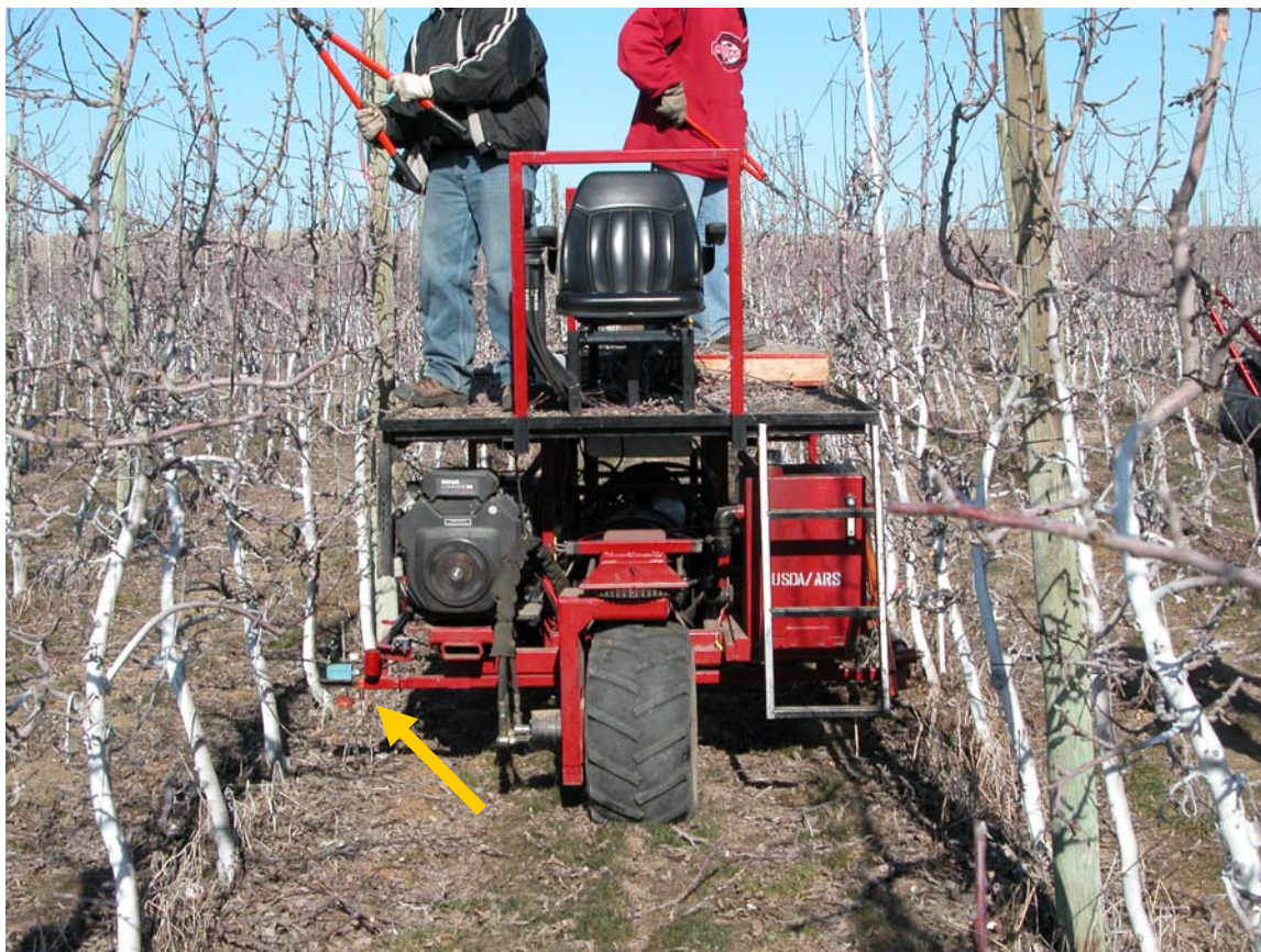
Figure 2. The modified Peterson machine being field trailed in 8 foot wide Braeburn block with actual row width at photo of less than 8 feet. The new adjustable row finding sensor is indicated at lower left.
