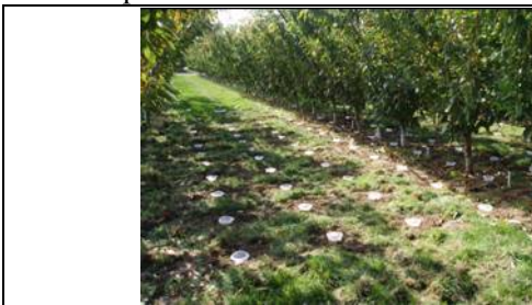
Figure 5. Catch can test arrangement in the cherry orchard.
