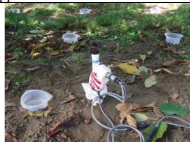
Figure 6. Flow and pressure meter test on a single nozzle.
