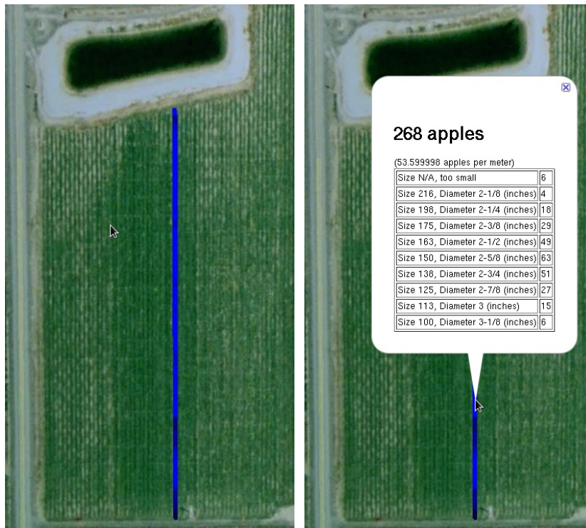
Yield map for a single row (left) and size information for a 16' section (right) for a green apple scan
