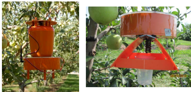
Figure 6: Modified zapper traps employing existing bucket trap (left) and delta trap (right) exterior designs.
