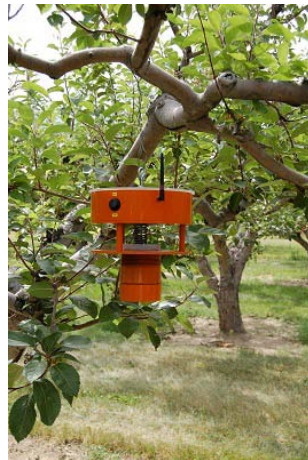
Figure 4: Second prototype model of the zapper trap (left); Second prototype of the zapper trap deployed in a WSU-TFREC orchard for field testing (right).
