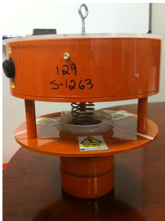
Figure 4: Second prototype model of the zapper trap (left); Second prototype of the zapper trap deployed in a WSU-TFREC orchard for field testing (right).
