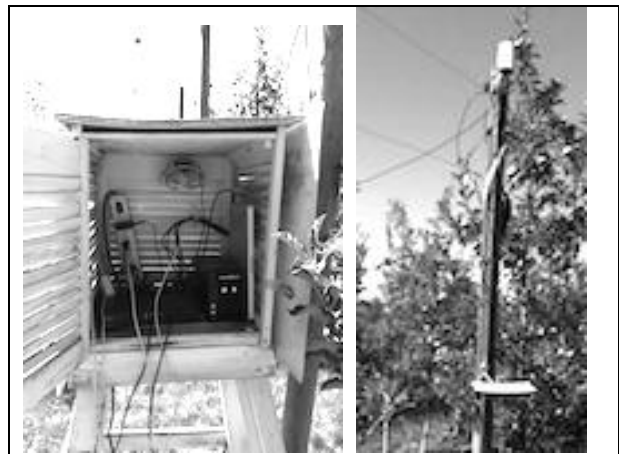
Fig. 1. Switch and hard-drive recorder with fan inside shelter and camera mounted above platform with attractant source.
