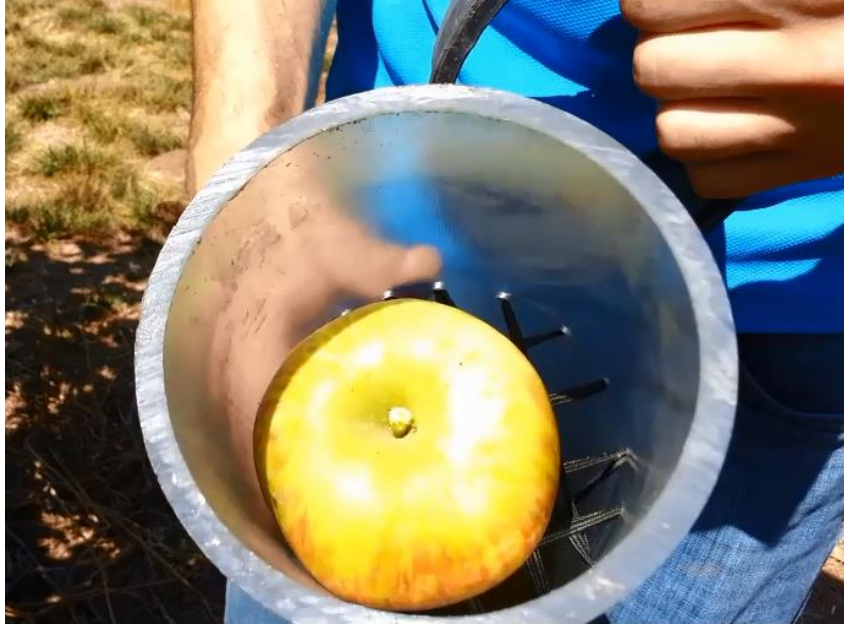
Figure 3 Vacuum tube showing elastic webbing in black and the apple captured by the webbing
