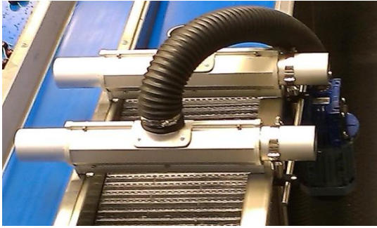
(a) Air Knife System Installed
