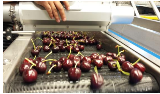
(b) Air knife System in Operation
