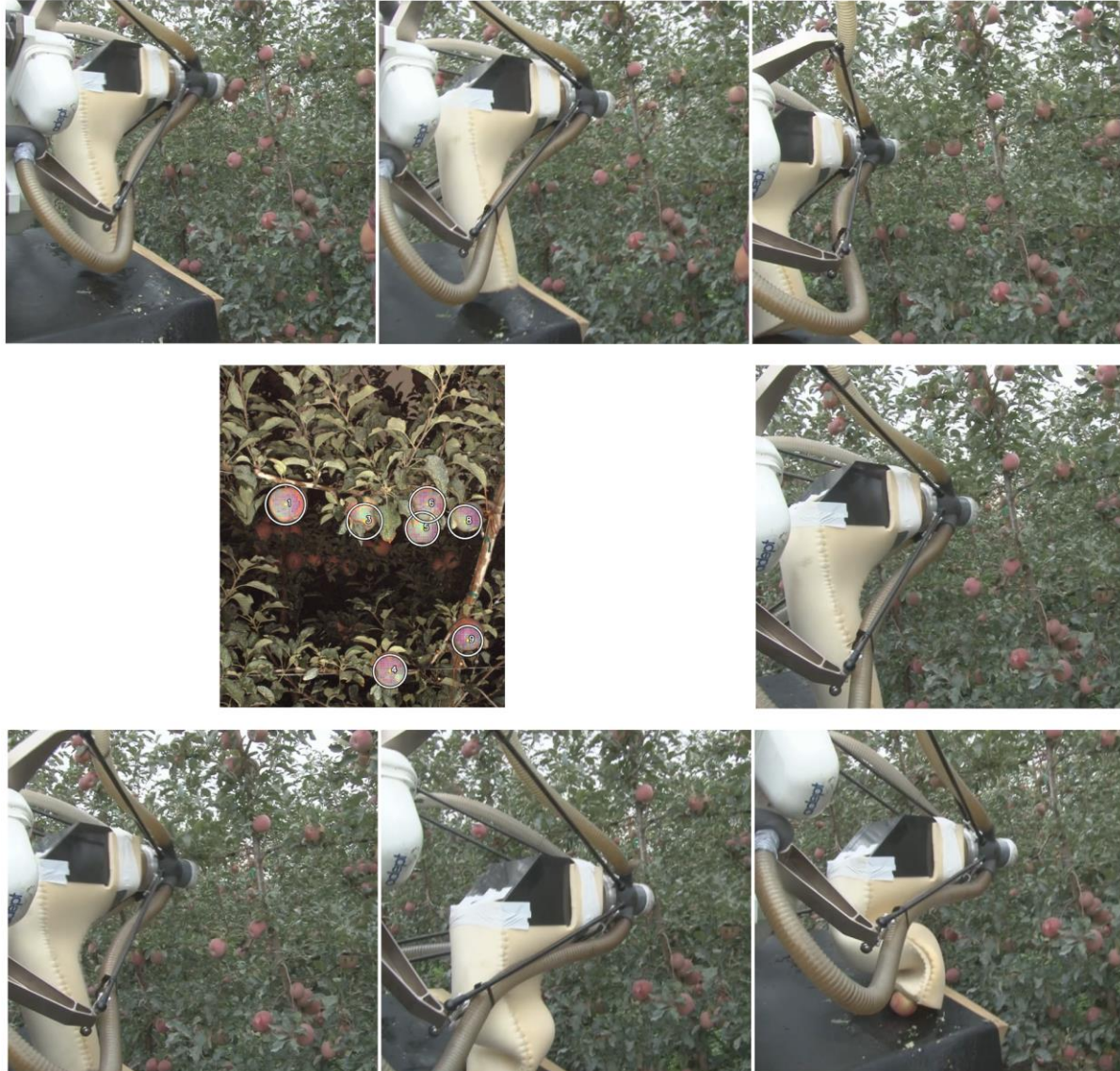
Figure 5 Frames of video capturing the pick events. The sensor output is shown in the center and the pick sequence is clockwise from the top left frame
