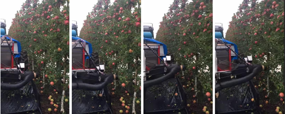
Figure 5 Image sequence of picking while continuously moving down the row
