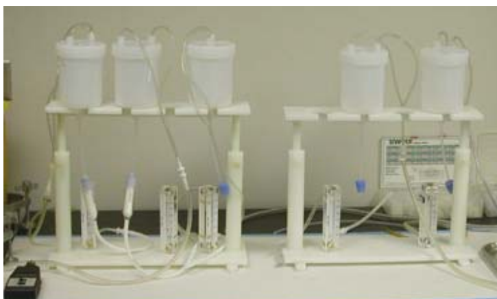
Fig. 1. Volatile trapping system for aged pheromone dispensers.
