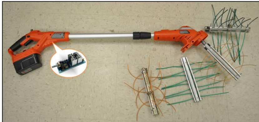
Figure 4. The second prototype of electrical powered with four thinning spindles and an electronic spindle speed controller
