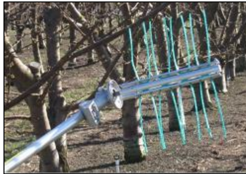
Figure 2. An example of thinning head design: with 2 trimmer lines of plastic covered wire of 6 inches long, and 8 strips in each line.
