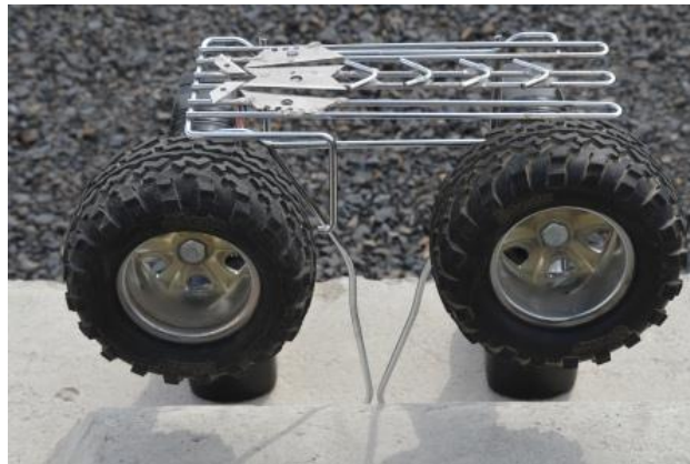
Figure 10 Wireframe separation barrier used for puncture reduction testing.
