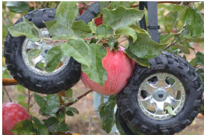
Figure 9. Prototype harvester wheel placement on an apple.
