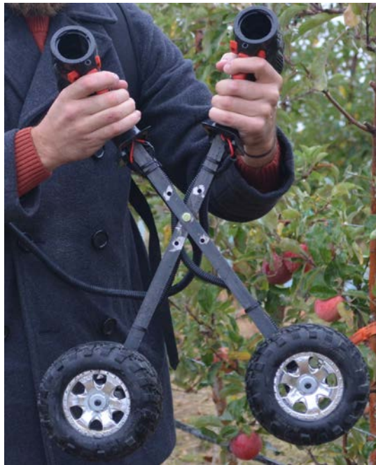
Figure 8 First apple twisting prototype (hand-held) built with rubber tires mounted to electric motors.
