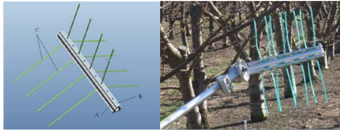
Figure 1. Examples of thinning spindle design: A 3D sketch (left) with 4 trimmer lines, eight 6 inches long strings in each line; and a thinning head (right) with 2 trimmer lines of 6 inches long plastic covered wire
