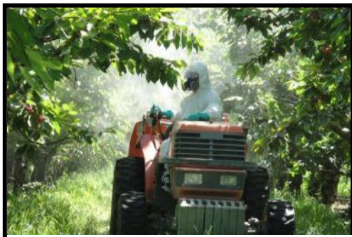
400 gallons/acre airblast spray application
