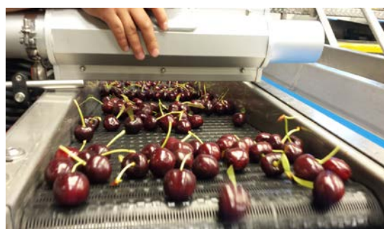
(b) Air knife System in Operation
