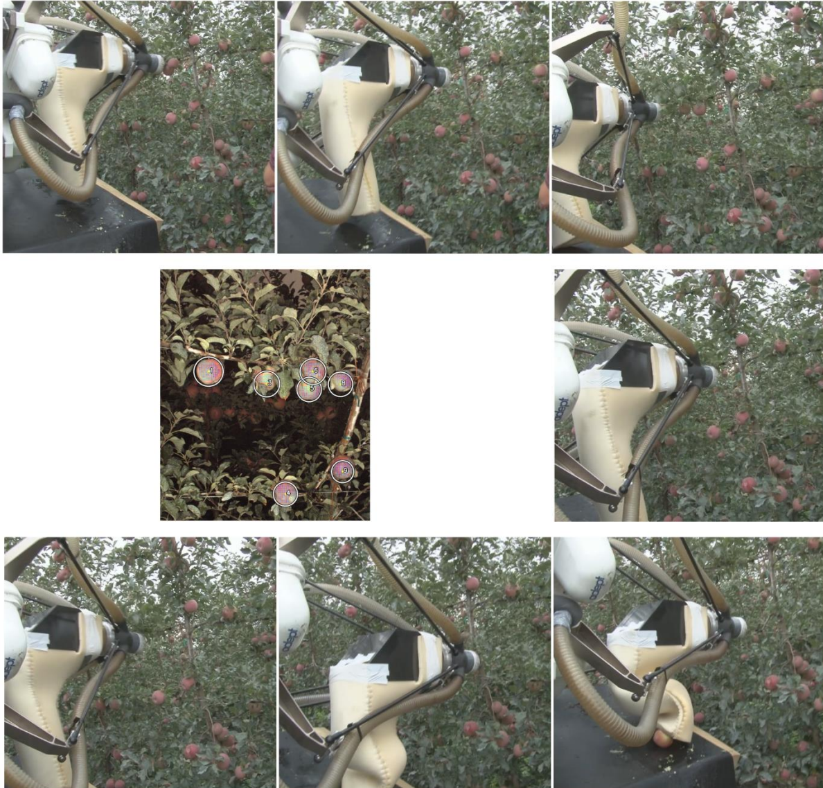
Figure 13 Frames of video capturing the pick events. The sensor output is shown in the center and the pick sequence is clockwise from the top left frame
