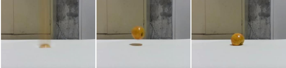
Figure 10 Drop testing of apples onto Memory foam. Left: Impact. Center: Rebound. Right: Resting Position.
