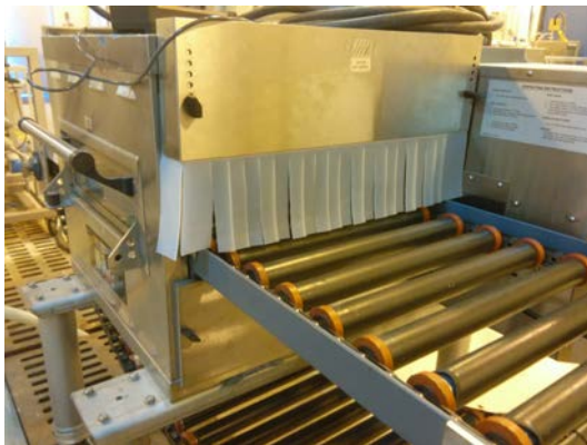
Fig 5. Slightly modified dryer (closed sides) and increased air flow speed by 20%
