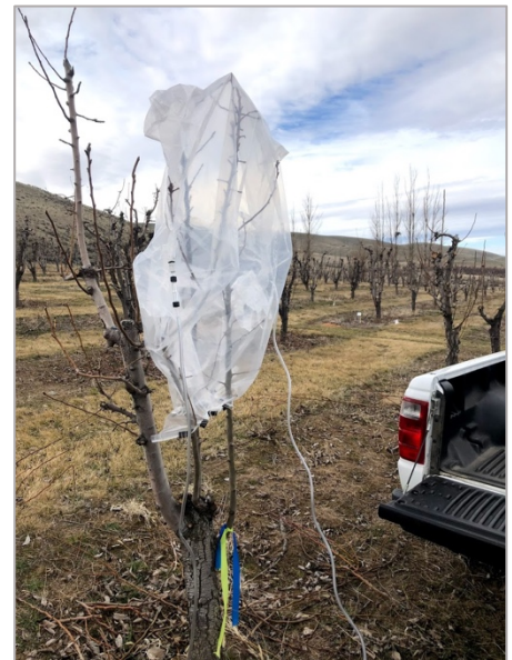
Figure 2. Example of volatile collection set up with a Bartlett pear tree at the USDA experimental farm in Moxee.
