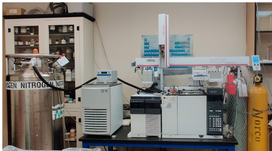
Figure 3. A GC-MS system used for in-situ volatile headspace analysis.
