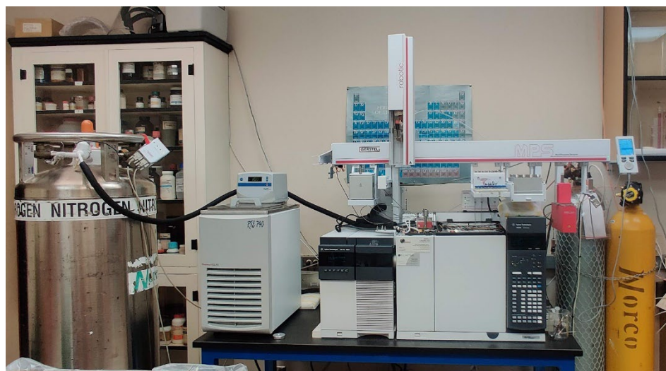
Figure 3. A GC/MS unit used for in-situ volatile headspace analysis.
