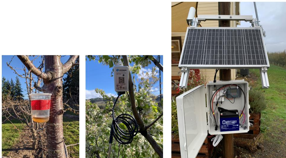
Figure 1. SWD trap, temperature sensor, and solar panel powered modem for data collection.
