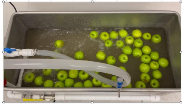
Fig. 1. An overview of the pilot dump tank used for testing.
