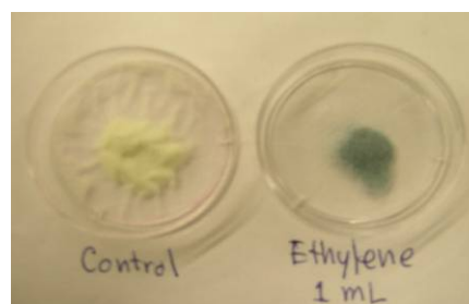
Figure 1: Palladium molybdate on activated silica gel with (right) and without (left) ethylene.
