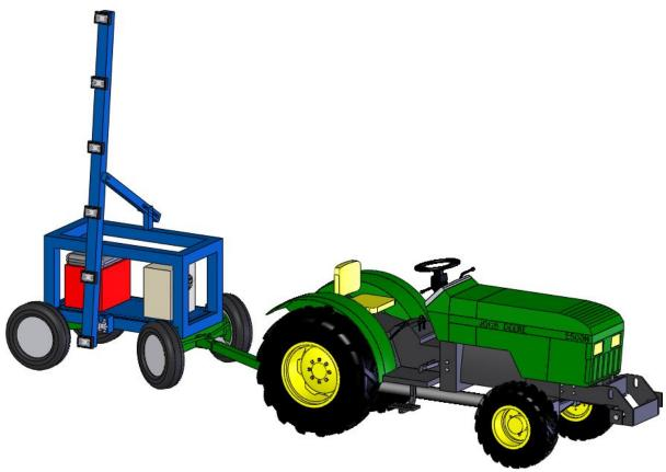
The *Scout* will be towed at a fairly constant rate of up to about .5 mph or .75 feet per second. The cameras will capture and record image data at 15 frames per second. This equates to an image every 0.6 inches, which is slightly more data than was used at the high-resolution scans in the 2007 project (one image every 2 cm or 0.79 inches).
