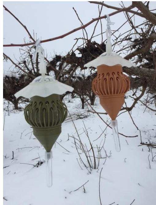
Figure 3. Prototype 3D-printed traps that capture winterform pear psylla directly into a preservative.
