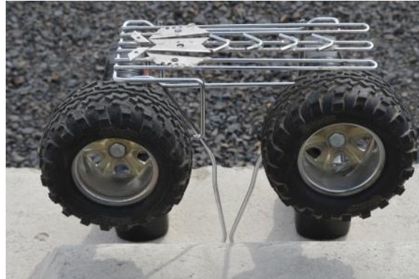
Figure 2 Wireframe separation barrier that minimizes rolling of apples over limbs.
