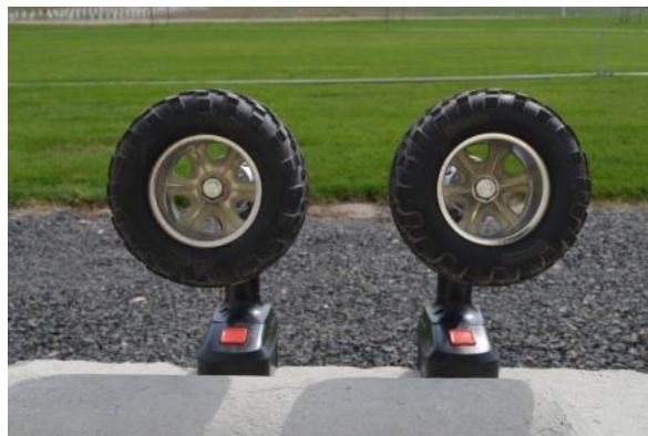
Figure 2 First apple twisting prototype was built with rubber tires mounted on electric hand drills.
