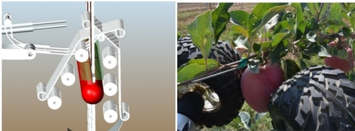
Figure 5 Proposed prototype apple harvester (left) and current testing module (right).
