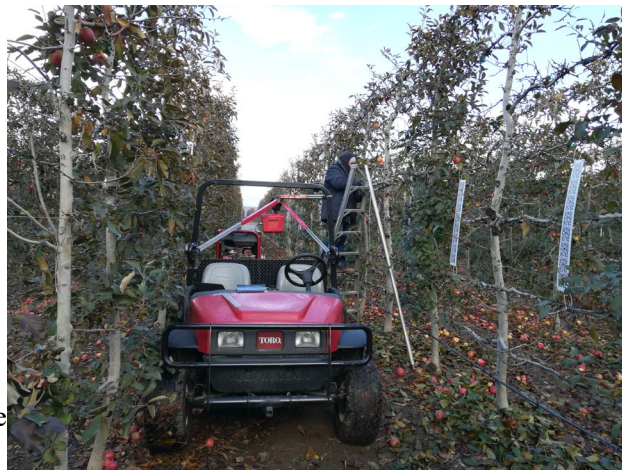
Fig. 2: Experimental setup during the field data collection. The active lighting camera was mounted on the back of the Gator.
