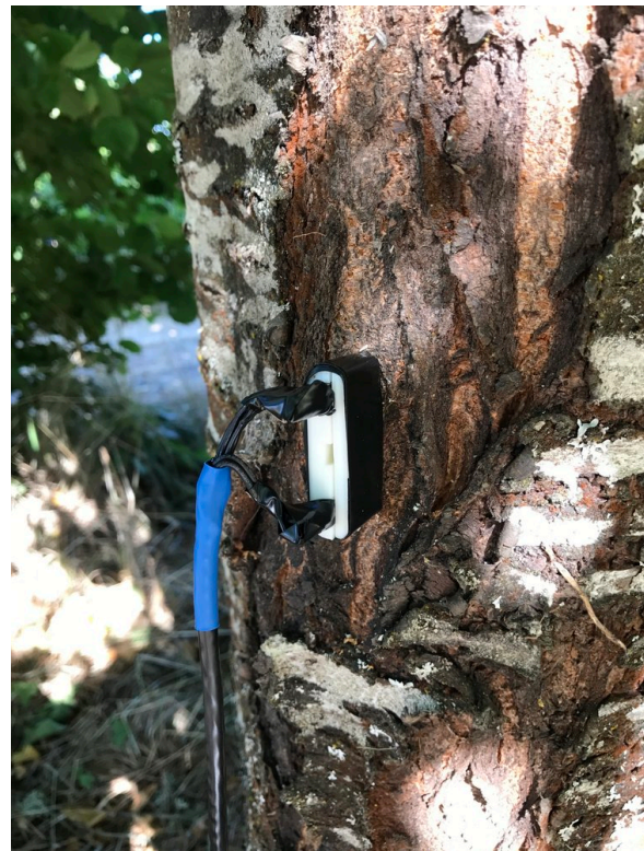
Figure 2: Sap flow probe deployed in a cherry tree August 2018
