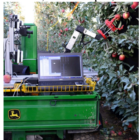
Fig. 1: A robotic system available to PI Karkee to carry out field evaluation of the pruning system
