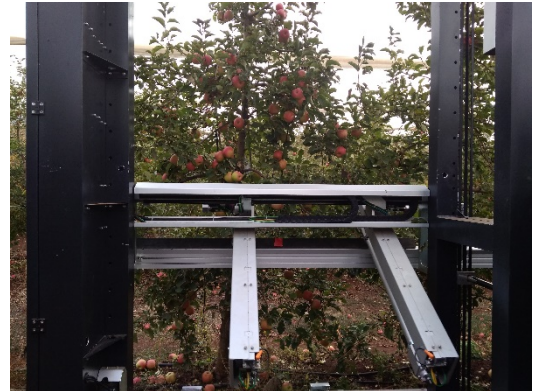
Fig. 1: Multiple robotic arms supported by one frame.
