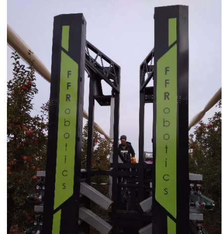
Fig. 4: One of the two full scale robotic harvester developed this year. This machine was fabricated in Israel and tested in 2018 harvest season.
