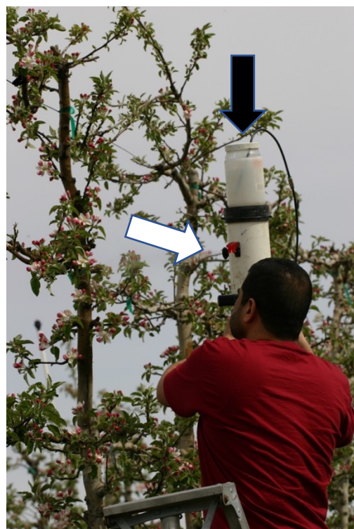
Figure 1. Single-nozzle electrostatic sprayer used for CNC applications to sweet cherry and apple trees. The black arrow indicates the 'tank' containing the CNC dispersion. The white arrow indicates the nozzle.
