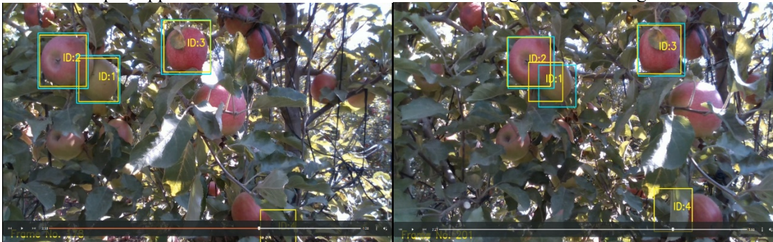
Fig. 3: Apple detection with changing viewing angle/direction. Some apples are more visible in the left image while others are so in the right image.
