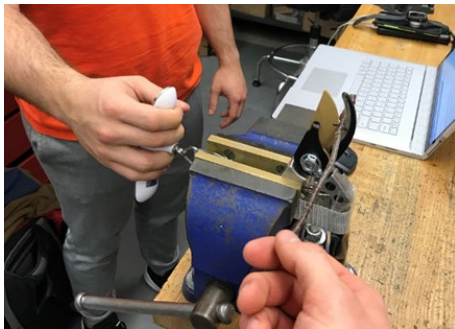
Fig. 6. Lab tests to determine branch cutting forces. Branches were collected from a commercial orchard in Prosser, WA in November 2018. Cutting tests used handheld shears and a force gauge.
