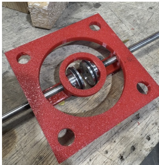
Subsequent Iteration with Cutting Blades for Stem Clipping
