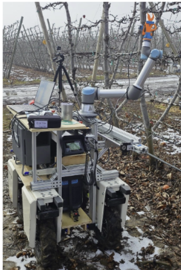
Figure 1. OSU's mobile orchard manipulation robot.
