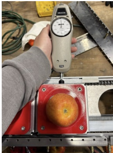
Test Setup for Clipping Force Measurement
