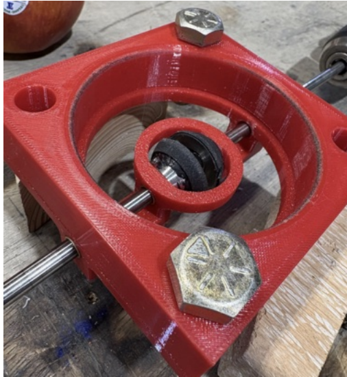
Early Iteration of Counter Rotating Concept, with Separately Driven Right/Left Rollers
