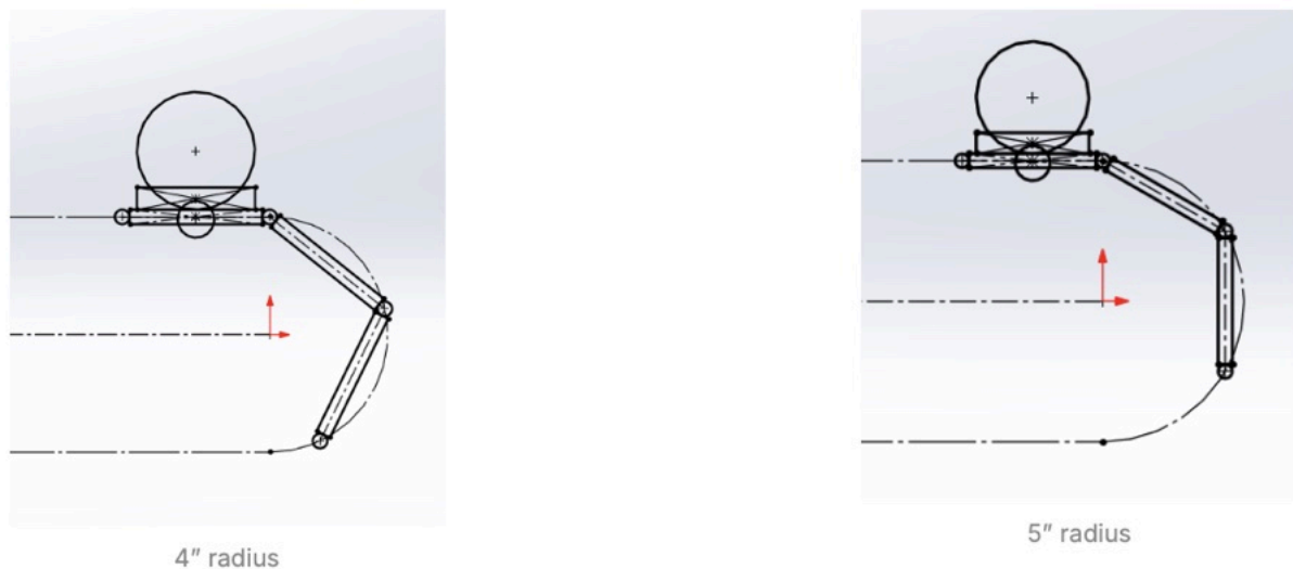
Layout Sketches for Various Alpha System Chain Pockets
