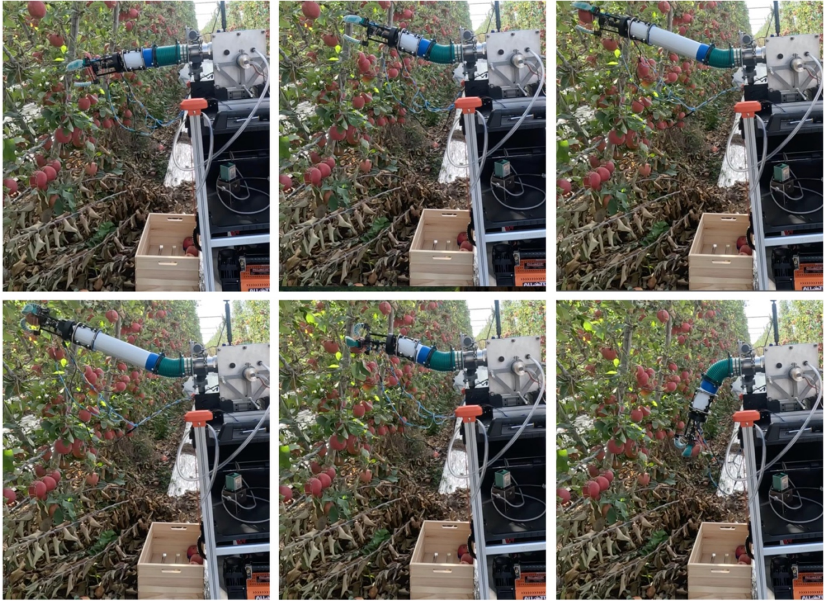
Figure.6 In the field study, one successful case involved the entire process: initialization, approaching, twisting, detaching, retracting, and dropping.
