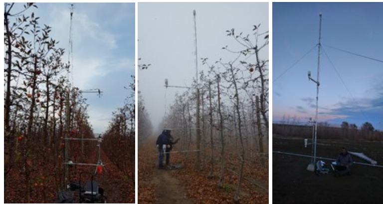
Fig. 5. Weather stations setup inside the field (left) MET 1 at 87' upwind from the edge of the orchard; (middle) MET 3 at 120' away towards the end of orchard from MET 1 in the same row; and (right) open field MET 2 at 600' downwind.
