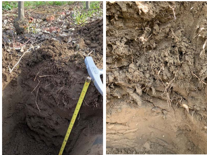
Figure 2. Soil profile for the top 3 feet. left: Site 1 (Quincy series) near Pasco, right: Site 2 (Warden series) in Sagemoor.
