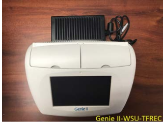
Figure 1. Portable Genie II instrument, battery-enabled acquired by Pathology lab at WSU-TFREC to be used LAMP detection of pathogens without prior DNA extraction.
