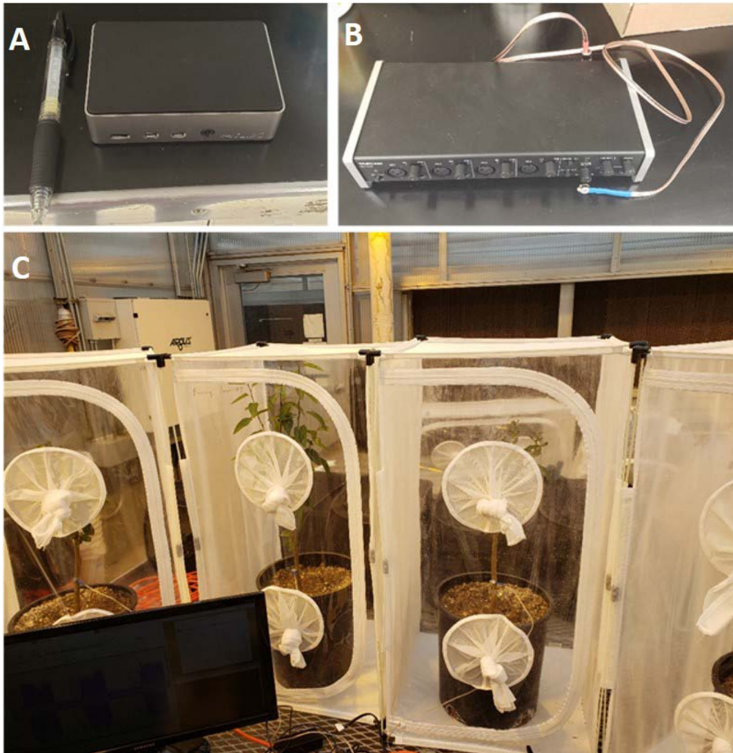
Figure 6. (A) raspberry pi computer for playing back signals. (B) audio interface with a playback device connected to the back. The LRA tip (blue tape) is attached to the stem of the plant to mimic vibrational communication. (C) Bugdorms set up with playback devices attached to the plants.
