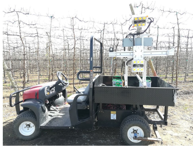
Fig. 4. A multi-view stereo camera system imaging dormant apple canopies. Camera system includes a linear slide.
