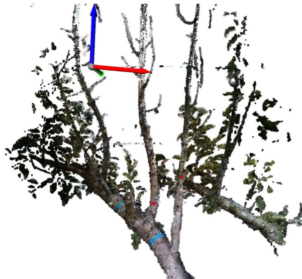
Fig. 5. A 3D point cloud of the tree structure generated by the Coordinated Depth Cameras system.
