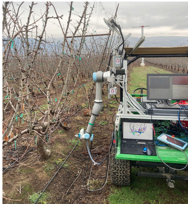
Fig. 8. The final pruning robot used for our 2021 evaluation, consisting of the UR-5e robot arm, the stereovision system, the Coordinated Depth Cameras system, and a custom electric pruning end effector.
