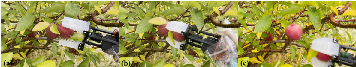
Figure. 17 Successful Apple Picking Process (a) Gripper Approaches Apple (b) Finger Contract around Apple (c) Gripper Pulls Away with Apple in its Grasp
