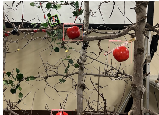
Figure. 15 One ZED 2 camera provided 3D position of target apples and 6 DoF (position and orientation) of the end- effector in global camera frame.
