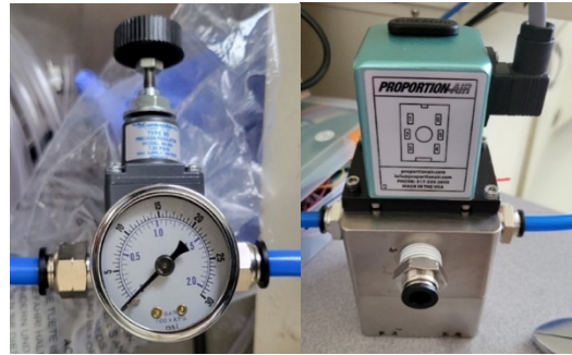
Figure 5 Hand Adjustable Pressure Regulator (Left) Digital Pressure Regulator (Right)
