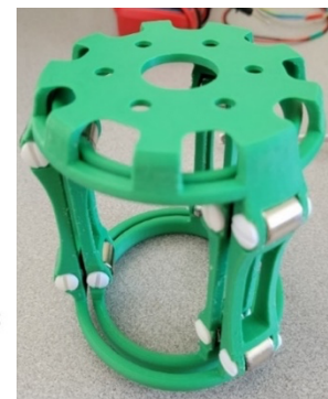
Figure 7 Labeled Component End-Effector Mount Diagram (Left) Physical 3D Printed End-Effector Mount (Right)
