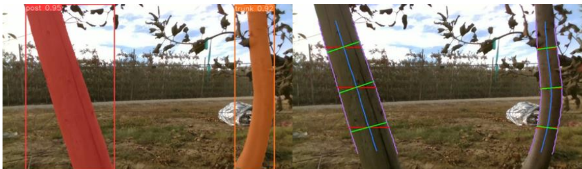
Figure 2. (Left) A typical segmentation of an image with a post and trunk. (Right) the width calculation method. The pink lines are the left and right sides of the object, the blue lines are the centerlines, the red lines are the initial width predictions, and the green lines are the corrected widths. The width is shown at three locations for illustration purposes.
