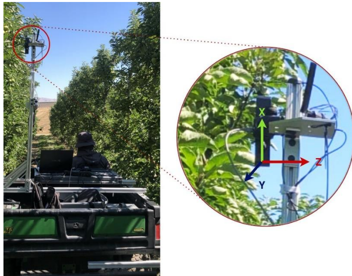
Figure 6. Data collection setup that includes a utility vehicle with Zed2i camera (Stereolabs, France) for image acquisition. The camera and its axes are zoomed in on the right.
