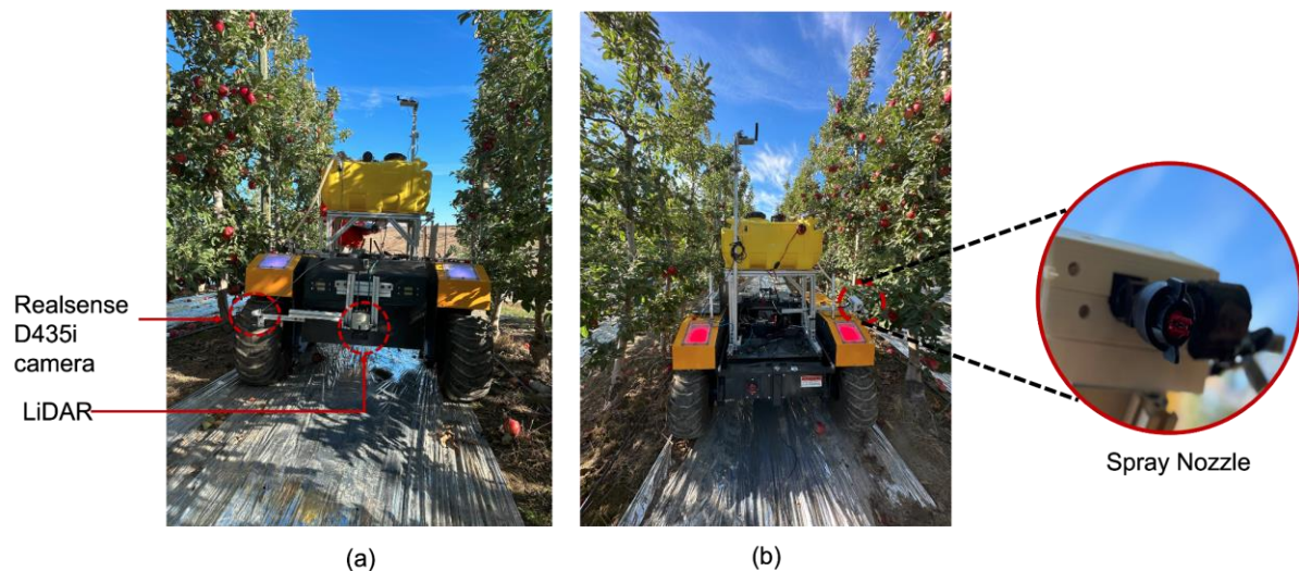
Figure 14: The integrated system: a) from front and b) from back. The front-facing LiDAR and the side-facing camera are visible in a), while the spraying nozzle has been zoomed in on b). The yellow tank on top contains the spray solution.
