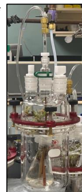
Figure 3. Example of volatile collection set up: 1L glass container with an inlet and outlet port so that volatiles can be collected using laboratory vacuum and onto charcoal collectors.
