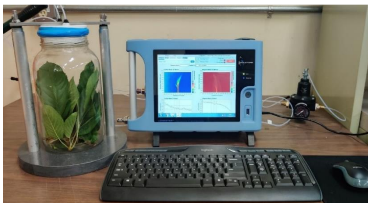
Figure 1. Portable FAIMS system analyzing cherry leaves volatile profile.
