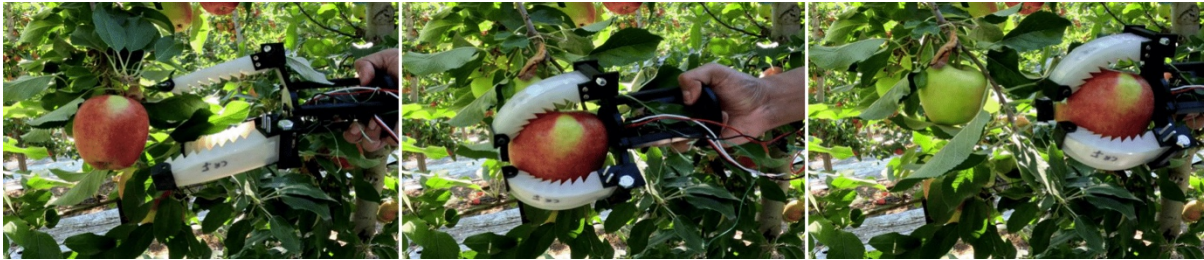
Figure 3. Gripper approaching, encompassing, and picking apple.
