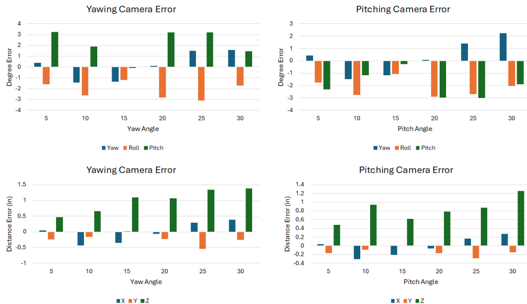
Figure 13. Error associated with pitch and yaw angle changes relative to row of apple trees.
